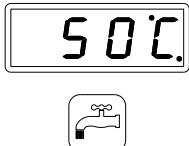
This light will go out when the DHW temperature is reached or the DHW demand is over.
