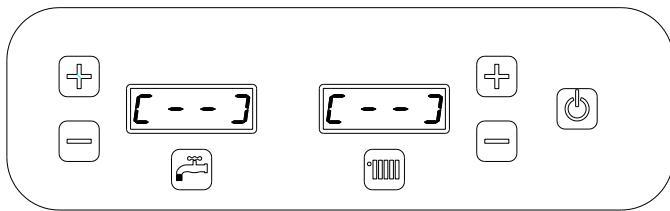
To unlock the buttons, press the same button down for a few seconds until the above displayed symbol goes off. If the boiler is disconnected from the mains or there is a failure in the house's electricity supply, the buttons will also be unlocked.
