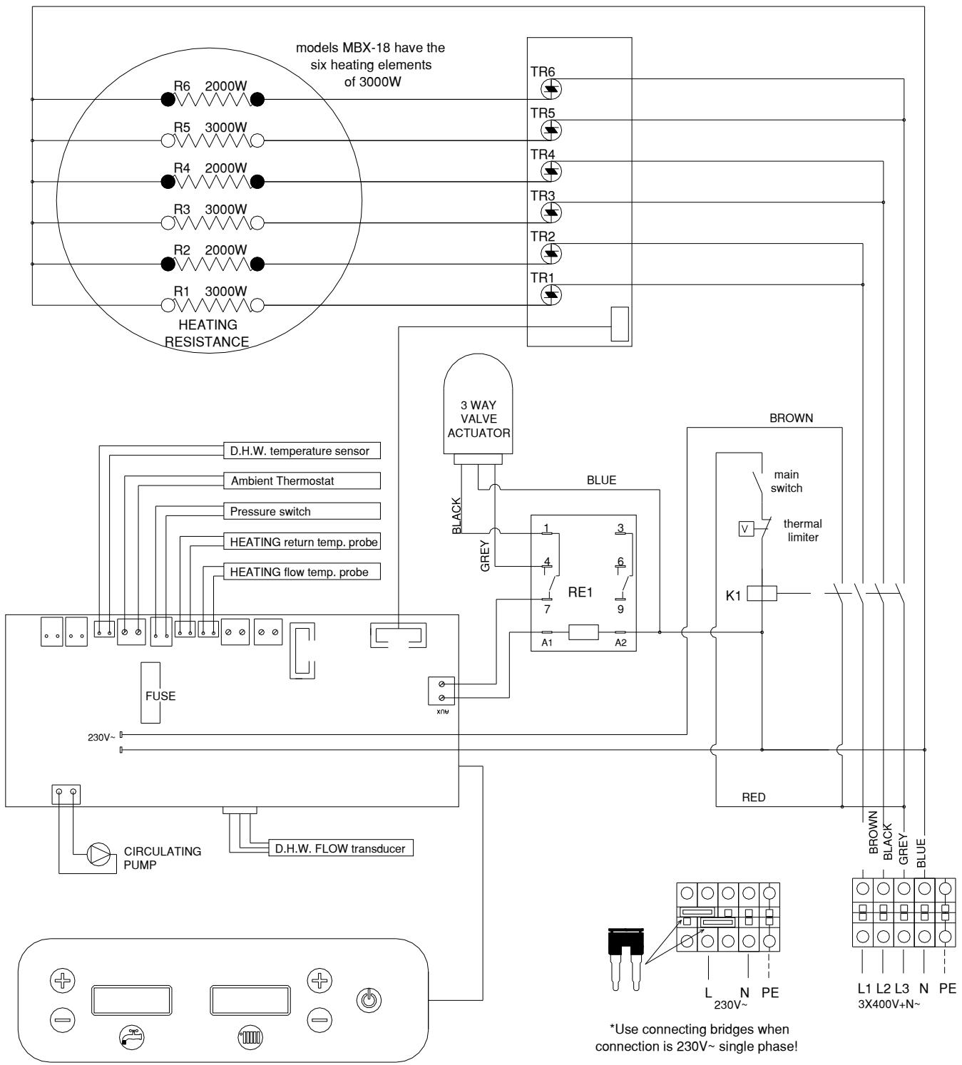
\*The standard configuration of the boiler only allows a maximum of 12kW when connected SINGLE-PHASE 230V~.
