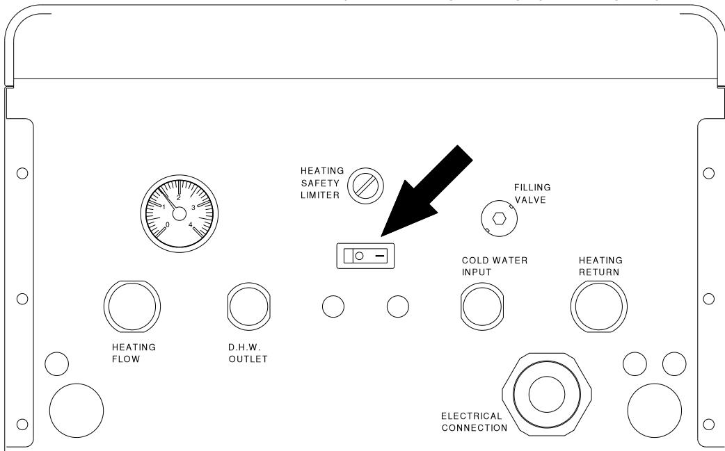
Unscrew & remove the black cap and push the small pin behind it until you hear a click. The limiter will not re-set until the temperature in the heating header drops below 100°C.
