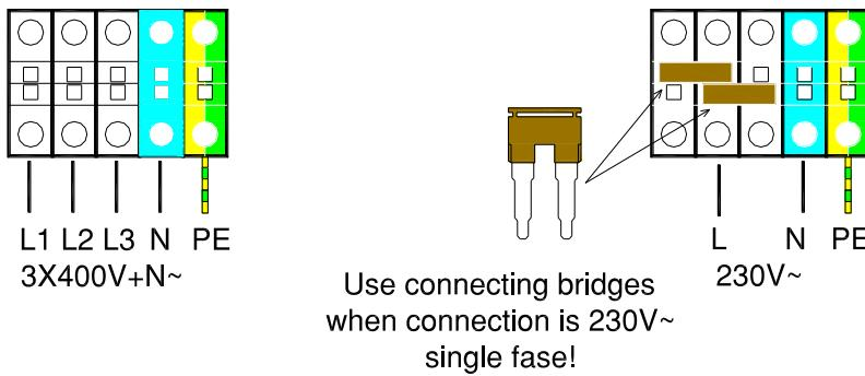
\* The standard configuration of the boiler only allows a maximum of 12kW when connected SINGLE-PHASE 230V~.
