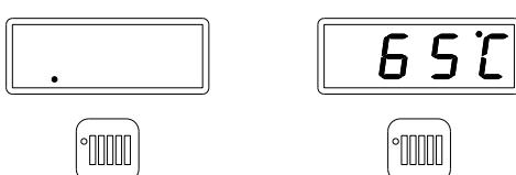
When the heating mode is selected the display will show the temperature of the heating water.
