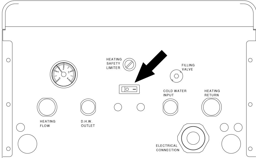
Turn on the boiler with the on/off switch located at the back of the boiler as shown.
