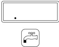
When the DHW mode is selected, the display will show the DHW temperature setting. The boiler will always give priority to DHW production over central heating.
